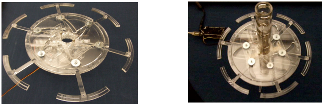
Figure 1. The left figure shows the Tangible Visualization Module (TVM) of the Weather Lamp. The right figure is the Weather Lamp with one module installed. A finished Weather Lamp will have three TVMs.
